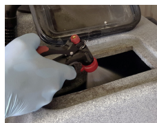
STEP 4 Clean recovery tank
