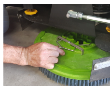
STEP 11 Remove brush from machine
