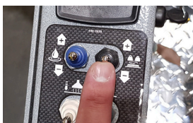
STEP 7 Adjust brush pressure
