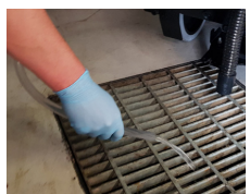
STEP 7 Empty solution tank
