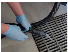
STEP 2 Empty recovery tank
