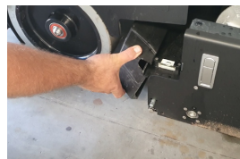
STEP 4 Empty Catchment Tray & push button to Check/Install brush
