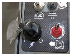
STEP 1 Switch off all functions
