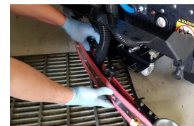
STEP 5 Check/Install squeegee
