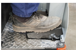
STEP 9 Press foot pedal to move forward
