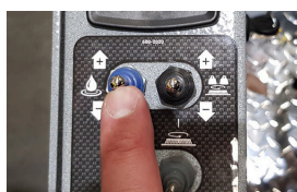
STEP 6 Adjust solution flow
