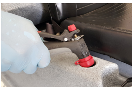
STEP 3 Fill the solution tank
