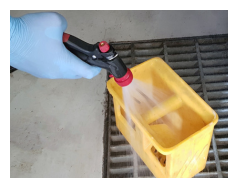
STEP 6 Clean drain saver
