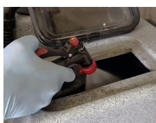
STEP 4 Clean recovery tank
