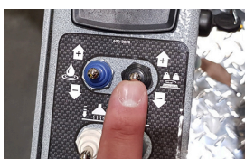
STEP 7 Adjust brush pressure
