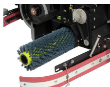
STEP 11 Remove brush from machine
