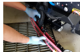
STEP 5 Check/Install squeegee
