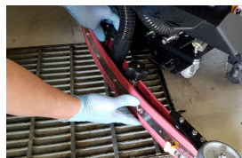
STEP 4 Check/Install squeegee
