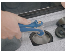
STEP 8 Clean solution tank
