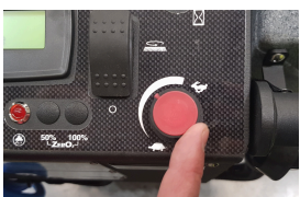
STEP 7 Adjust speed control
