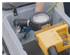
STEP 4 Clean recovery tank
