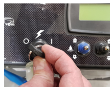
STEP 1 Switch off all functions
