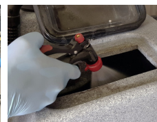
STEP 4 Clean recovery tank
