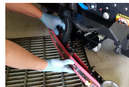
STEP 5 Check/Install squeegee
