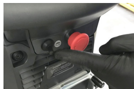
STEP 4 To release brush/pad toggle switch twice
