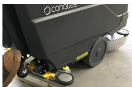
STEP 7 Use foot to depress level at rear of machine to lower brush
