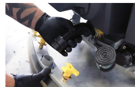
STEP 5 Check/Install squeegee
