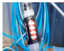
STEP 10 Indicator will stop spinning once full
