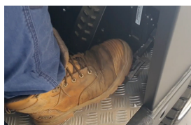
STEP 10 Depress accelerator pedal to move and control speed
