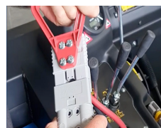
STEP 11 Plug in to charge for minimum of 8 hours
