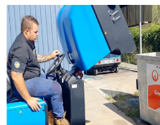
STEP 5 Position hopper over waste receptacle
