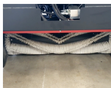
STEP 7 Ensure broom is free from strapping
