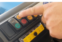
STEP 8 Start fan. Fan MUST be running while sweeping
