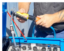
STEP 9 Connect Battery Fill Gun to a standard hose
