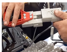
STEP 9 Plug into charger if battery is below 20%
