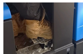
STEP 10 Depress upper pedal for forward, lower for reverse
