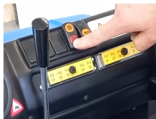
STEP 3 Activate filter shaker
