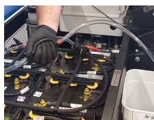
STEP 11 Top up fluid with distilled water
