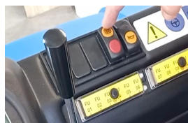
STEP 7 Turn on vacuum. DO NOT operate in wet conditions
