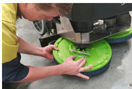
STEP 3 Check/Install pad
