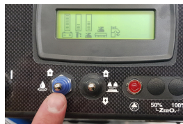
STEP 5 Adjust solution flow
