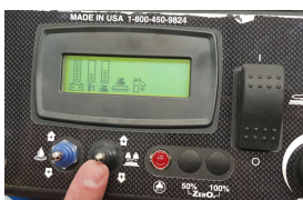
STEP 6 Adjust pad pressure
