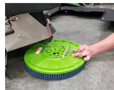
STEP 11 Remove pad from machine
