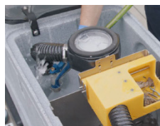
STEP 4 Clean recovery tank
